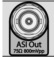
Figure 2-16. DVB ASI Out BNC Connector for BER Measurements (Option 57 and Option 79)
